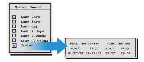
Selecting any of the other options and pressing **Enter** starts playback and displays the **Motion Search Setup Screen**.
